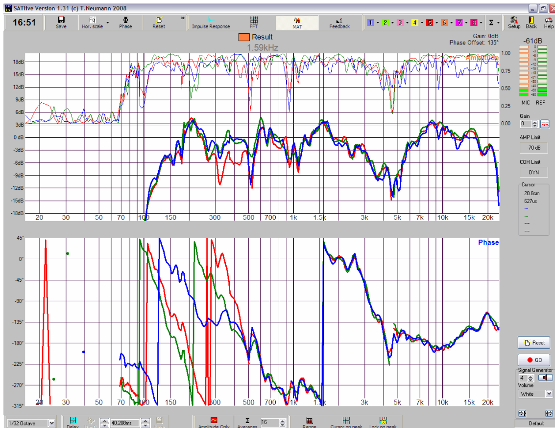
Fig 19. Both delay settings improve the magnitude frequency response with respect to initial configuration without delay.
