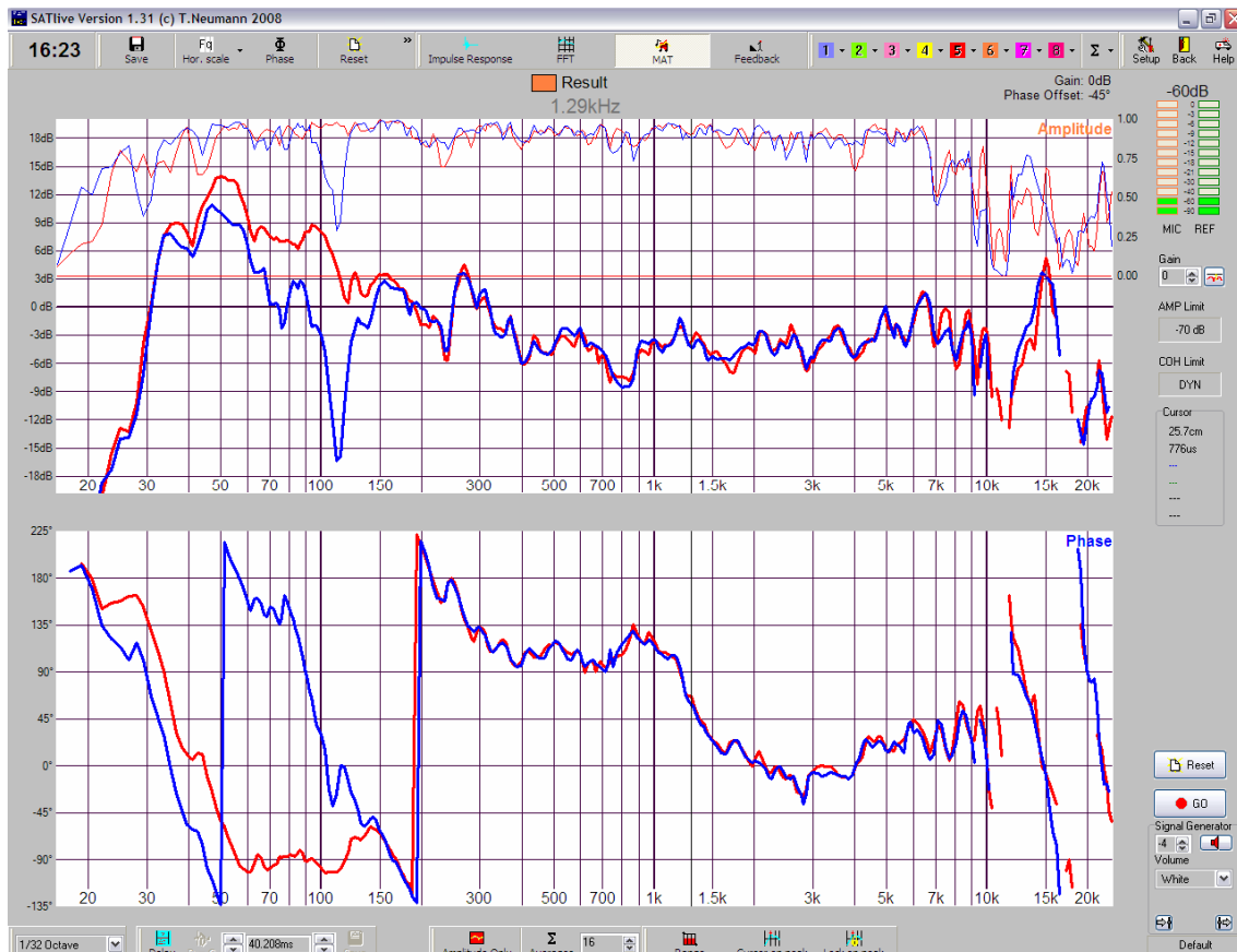
Fig 24. Magnitude frequency response before (blue trace) and after (red trace) phase alignment.
