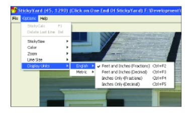
This function allows the user to make two decisions. Firstly, you can convert your English measurements to Metric and your Metric measurements to English. It also allows the user to choose which increments will be displayed: feet and inches using fractions, feet and inches using decimals, inches only with fractions, inches only with decimals, centimeters only or meters and centimeters.
