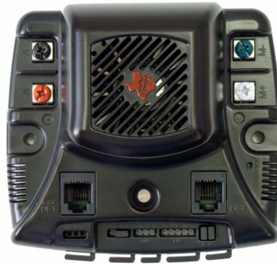
Figure 2. MDL-BDC24 Motor Control Module
