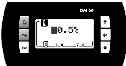
View and/or modify the offset, or set point, of the temperature control desired for the Unit selected.
