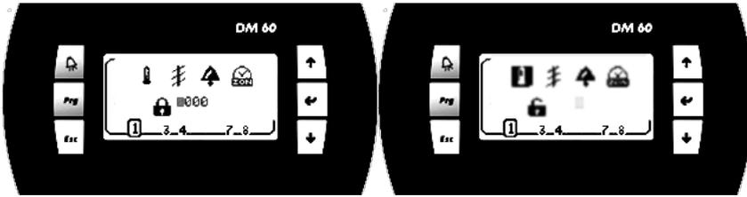
Access to the setup menus is protected by a password.
