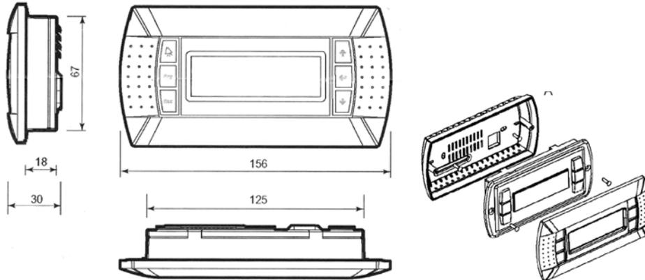
The optional DM60 delivered is designed to be wall mounted.
