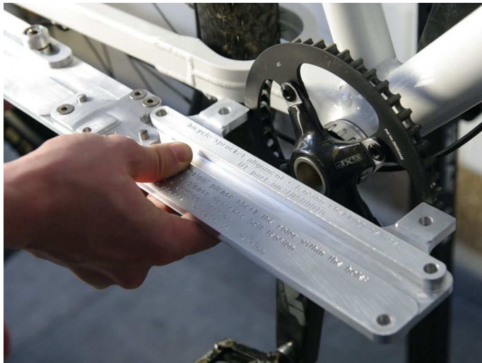
fig 8: belt line alignment via bottom bracket spacer
