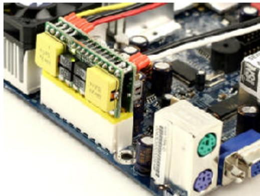
Note: power consumption as low as 9 W has been recorded with hard disk, graphics card (ATI 9250) all running with a reasonable amount of usage but without heavy 3D running. Those numbers have to be confirmed officially.
