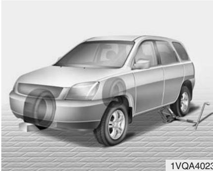
4. Remove the wheel lug nut wrench, jack, jack handle, and spare tire from the vehicle.
