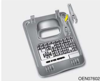
3. Pull the suspected fuse straight out. Use the removal tool provided in the fuse panel cover.
