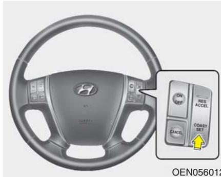
3. Push the COAST/SET switch, and release it at the desired speed. The SET indicator light in the instrument cluster will illuminate. Release the accelerator at the same time. The desired speed will automatically be maintained.
