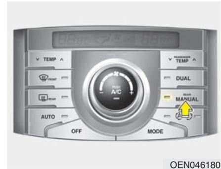
The temperature, fan speed and mode of the rear climate control system can be controlled independently regardless of the front climate control system operation.
