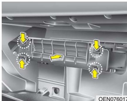
3. Remove the climate control air filter case pulling out both sides of the cover.
