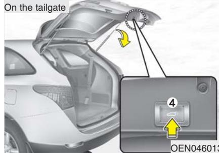
The power tailgate can be opened and closed automatically with the transmitter (or smart key), the main control button on the driver side crash pad, or the sub control button or handle switch on the tailgate.
