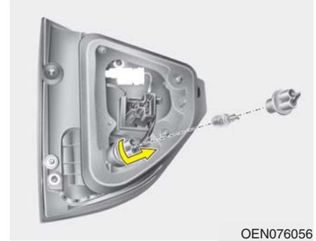
7. Insert a new bulb by inserting it into the socket and rotating it until it locks into place.
