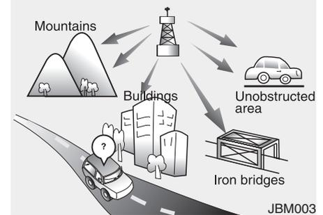
FM broadcasts are transmitted at high frequencies and do not bend to follow the earth's surface. Because of this, FM broadcasts generally begin to fade at short distances from the station. Also, FM signals are easily affected by buildings, mountains, or other obstructions. These can result in certain listening conditions which might lead you to believe a problem exists with your radio. The following conditions are normal and do not indicate radio trouble:
