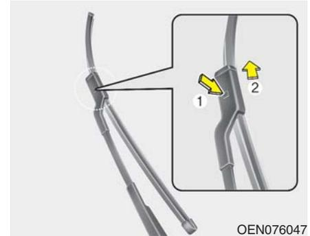
4. Press the button and slide the blade assembly upward.
