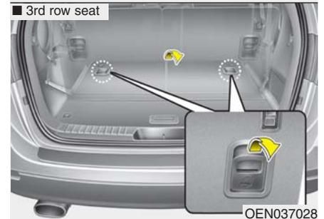
4. Pull on the seatback folding lever, then fold the seat toward the front of the vehicle. When you return the seatback to its upright position, always be sure it has locked into position by pushing on the top of the seatback.
