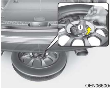
4. After the spare tire reaches the ground, continue to turn the wrench counterclockwise, and draw the spare tire outside. Never rotate the wrench excessively, otherwise the spare tire carrier may be damaged.
