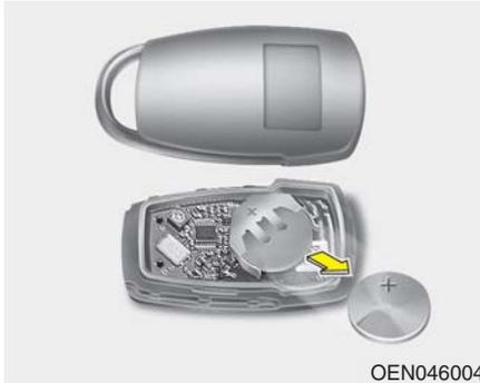
2. Replace the battery with a new battery (CR2032). When replacing the battery, make sure the battery positive “+” symbol faces up as indicated in the illustration.
