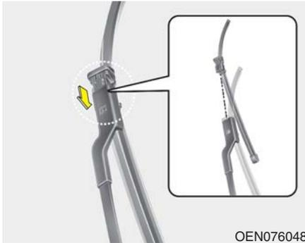
5. Install the blade assembly in the reverse order of removal.
