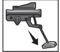
The trolley will reconnect on the next time the opener is activated.
