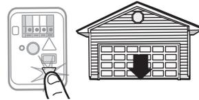
**NOTE:** The UP and DOWN Buttons can be used to move the door up and down as needed.
