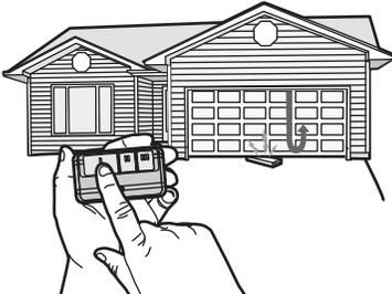
If the door stops and does not reverse on the obstruction, increase the down travel (see Adjustment Step 1).
