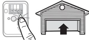
**NOTE:** The UP and DOWN Buttons can be used to move the door up and down as needed.
