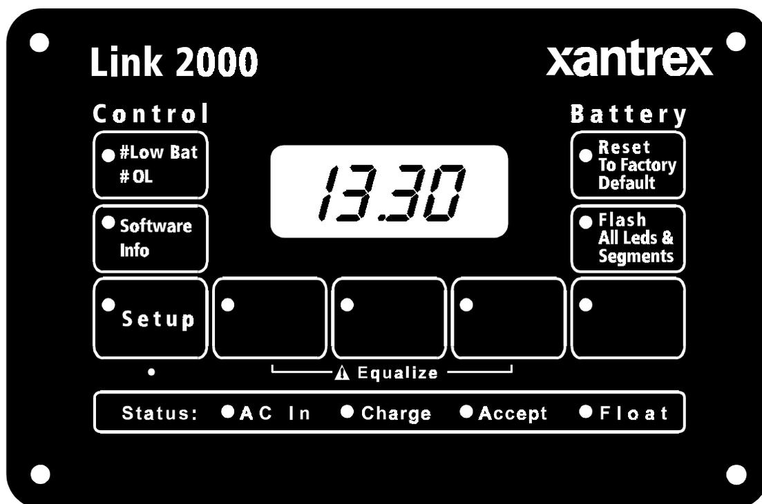
**# LOW BAT/ # OL:** The number of Inverter Low Battery shutdowns (since last reset) is displayed with a minus sign (negative number). The number of Inverter shutdowns (since last reset) from other causes are displayed with no sign (positive number). The display alternates at three-second intervals until the button is released.
