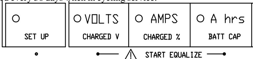
**CAUTION! Turn off voltage sensitive DC loads before equalizing battery!**
