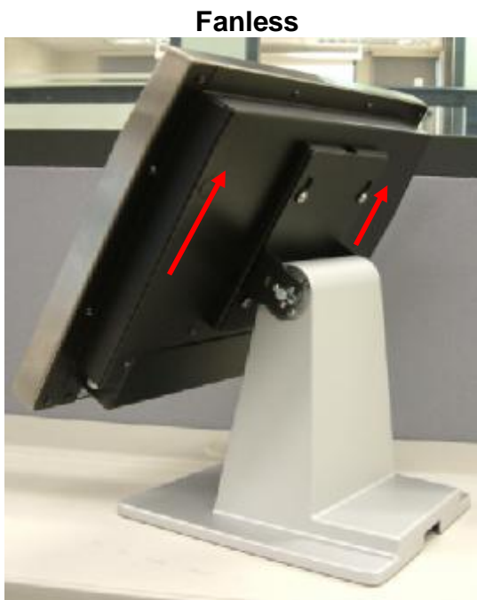
b. Lift the panel up and separate it from the stand bracket
