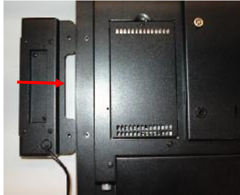
b. slide the MSR into the position
