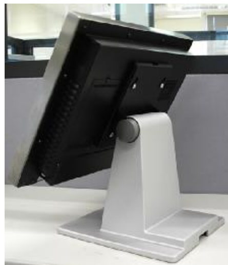
f. Attach the hinge covers(2) to finish the installation
