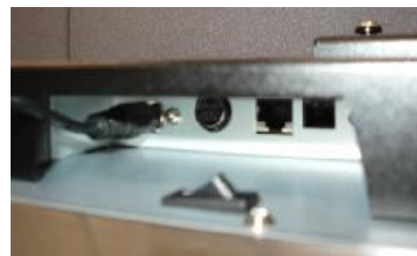
e. Connect the MSR cable to the PS2 socket to finish the installation
