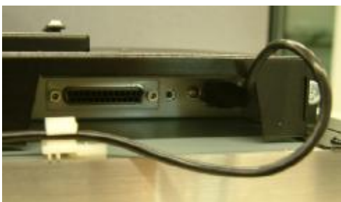
e. Connect the MSR cable to the PS2 socket to finish the installation
