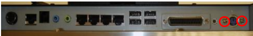
c. Remove the hex screws (2) to replace the main board
