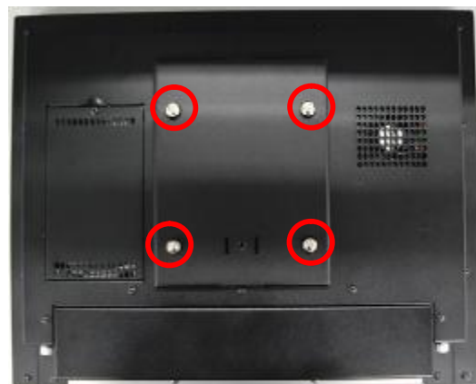
c. Attach the panel bracket to the VESA holds and tighten the screws (4)
