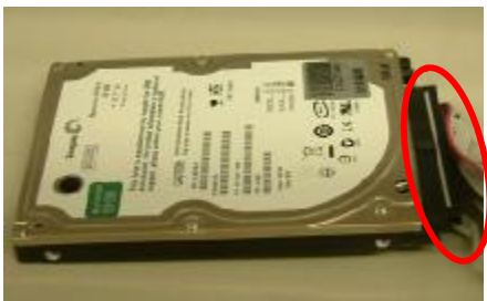
b. Disconnect the IDE cable from the HDD
