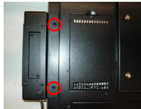
c. Tighten the screws (2)
