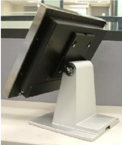
d. Attach the panel to the stand bracket
