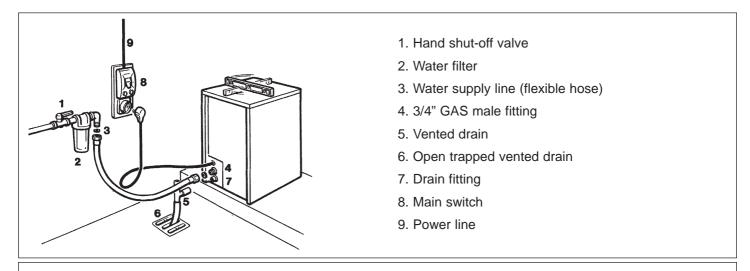
WARNING This icemaker is not designed for outdoor installation and will not function in ambient temperatures below 10°C (50°F) or above 40°C (100°F). This icemaker will malfunction with water temperatures below 5°C (40°F) or above 40°C (100°F).
