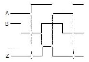
Figure 6-2: Timing diagram for digital encoder signals
