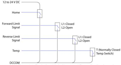
Figure 6-3: Equivalent Limit, Home, and Temp circuit schematic
