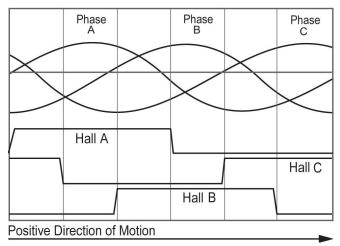
Figure 6-1: Motor Phase and Hall Sensor Timing
