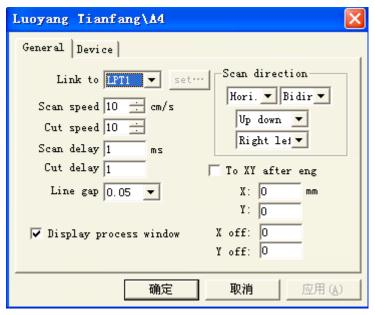
**Link to•••**: The direction of engrave machine and computer connection.
