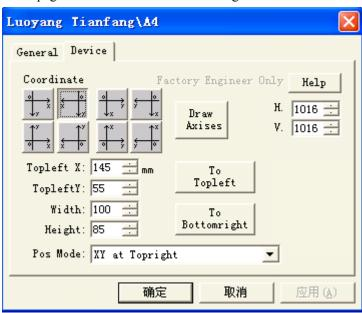
**Help**: It's showing the method of coordinates direction, topleft corner coordinate and engrave width. If the methods not clear you may test according to the steps of explanation.
