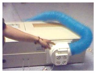
Switch on fan while run the machine now you can switch on the machine and try to make a small sample of the engraving. When you run the machine, make sure the water pump is always running and the water on pipe is circulatory flowing!
