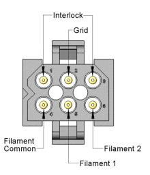
Base connections of AIG1x gauges.
