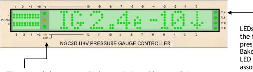
The units of the pressure display are indicated by one of three LEDs in the display area. The centre orange LED indicates that mBar has been selected, the green LED above it indicates Pascal and the green LED below indicates Torr.
