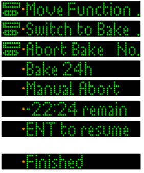
Start Bake by turning the Function Switch to BAKE and press ENT.
