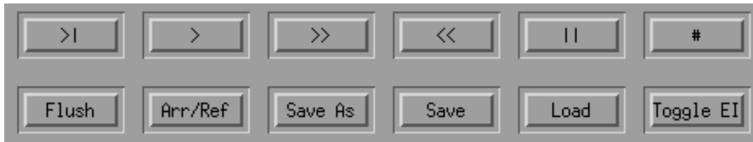
Figure 3.9: The buttons that control the tool. Top row (from left to right) : One Step, Run, Fast Forward, Rewind, Pause and Abort. Bottom row : Flush the cache, (coloring by) Array Ref ID or Array ID, Save As status file, Save status file, Load status file and Toggle Extra Info
