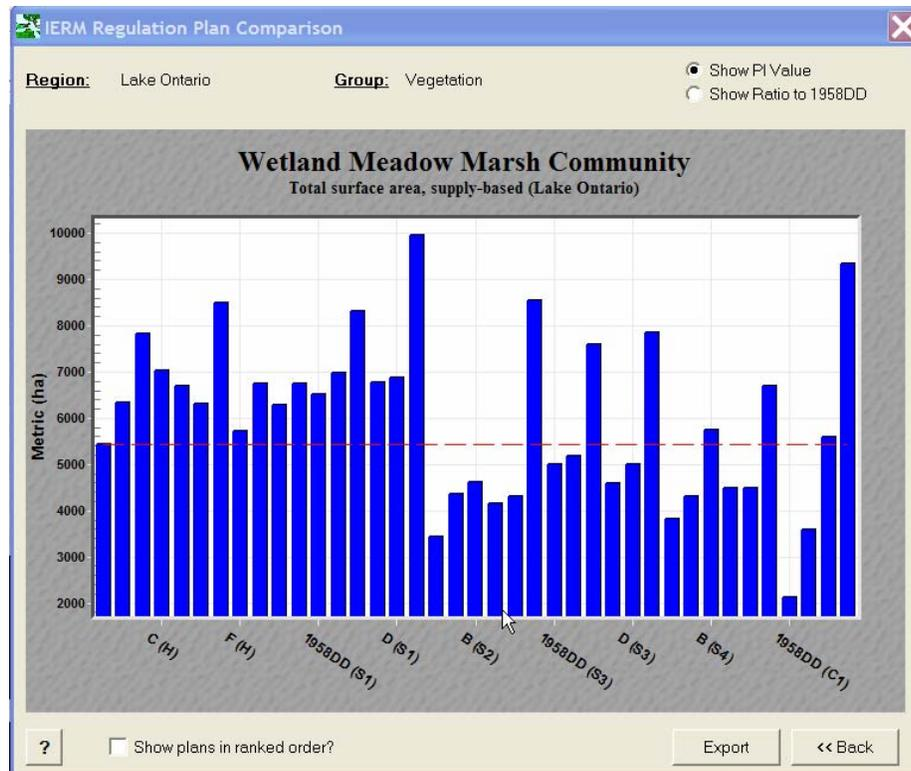
**Figure 3-10. Plan Comparison Visualization**
