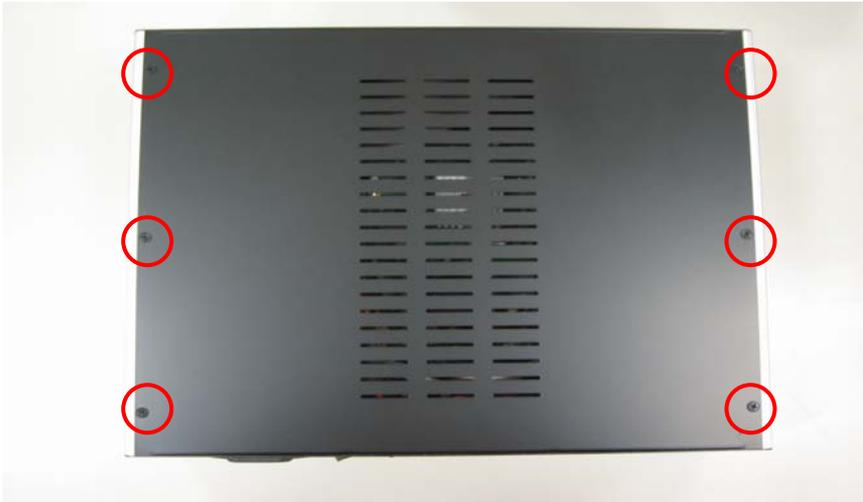
3. Unscrew four screws from front and back panel
