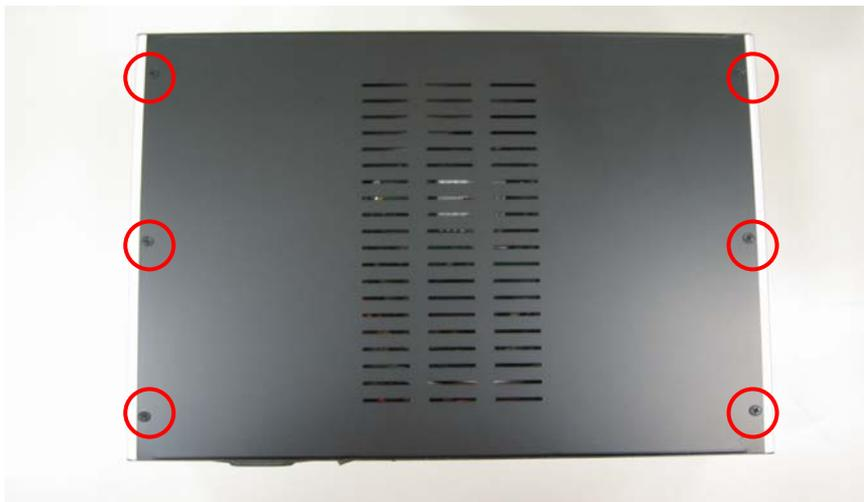
6. Unscrew the four screws from front panel and back panel
