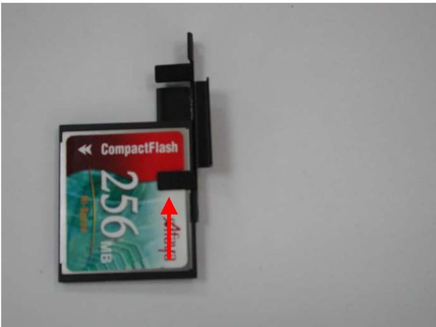
5. Inserting the CF carrier back and assembling with 2 screws to CF door located on rear panel.
