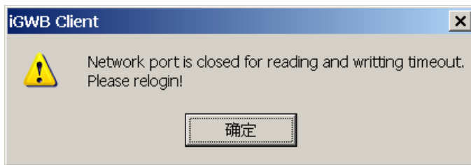
Figure 4-4 Prompt message of bill console in case of a network failure
