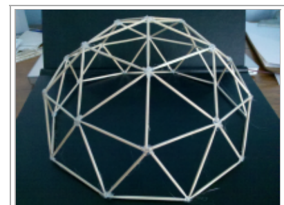
2V/L2 Icosahedral Dome Completed Concept
