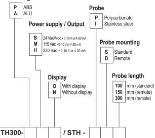
Example : TH300-PBN/STH-PD300 = humidity transmitter type TH300, with ABS housing, 24 Vac/Vdc power supply, without display, with polycarbonate remote probe length 300mm.
