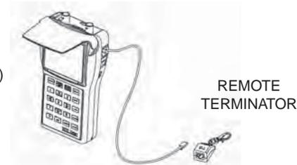
**Select UTP Cable Test mode:** Press the "3" key to enter the UTP test mode.
