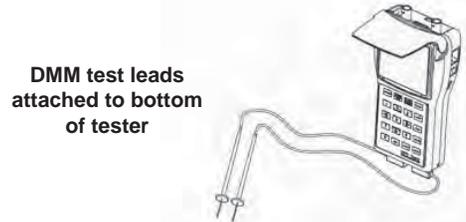
**Select Multimeter mode:** Press "6" on the keypad to turn ON the DMM (digital multimeter).
