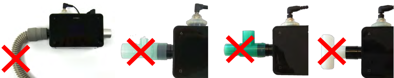
Worse set up: Kink, T-piece, elbow-piece etc. at gas inlet
