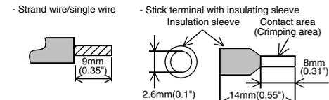
When using a stick terminal with insulating sleeve, choose a wire with proper cable sheath referring to the above outside dimensions, or otherwise, the wire cannot be inserted easily.
