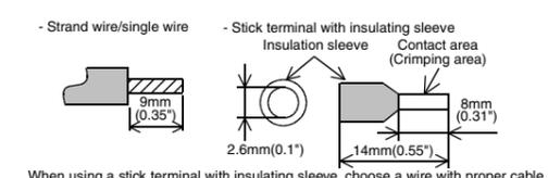
When using a stick terminal with insulating sleeve, choose a wire with proper cable sheath referring to the above outside dimensions, or otherwise, the wire cannot be inserted easily.
