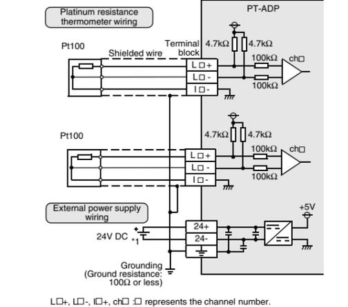
\*1 24V DC service power supply of the FX3U Series PLC can also be used.
