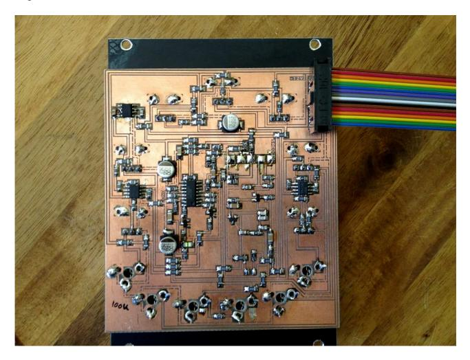
Mount the other end of the power cable to the powerboard of your Eurorack case. Make sure, that pin 1 is connected to -12 volt.
