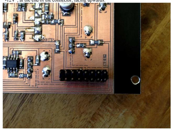
This is pin 1, and the -12 volt from your Eurorack power board, should be connected to this pin.
