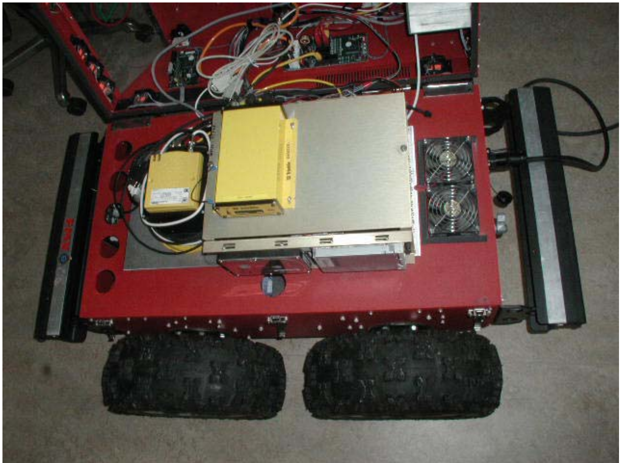
Figure A.2. This picture shows the ATRV with its lid open. The box in the center is the computer and the black box in front of it is the inertial sensor.
