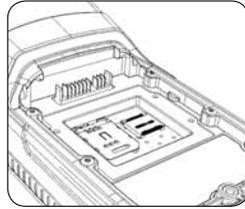
7 Close the microSD card door and slide it towards the bottom of the computer to lock it in place.
