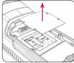
5 Slide the microSD card door towards the top of the computer to unlock it and open the door.
