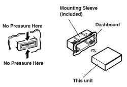
Remove the Detachable Front Panel (refer to page 5). Slide mounting sleeve from main unit. (see "Removal" on this page).
