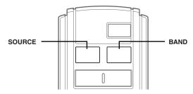
Press the BAND button on the CDA-9827/CDA-9826/ CDA-9825 or the RUE-4187 to activate the CD Changer Selection mode. 3 The CD Changer Selection mode remains active for 8 seconds after step 2 is performed. Press the BAND/TEL. button until the desired CD Changer indicator appears on the display.
