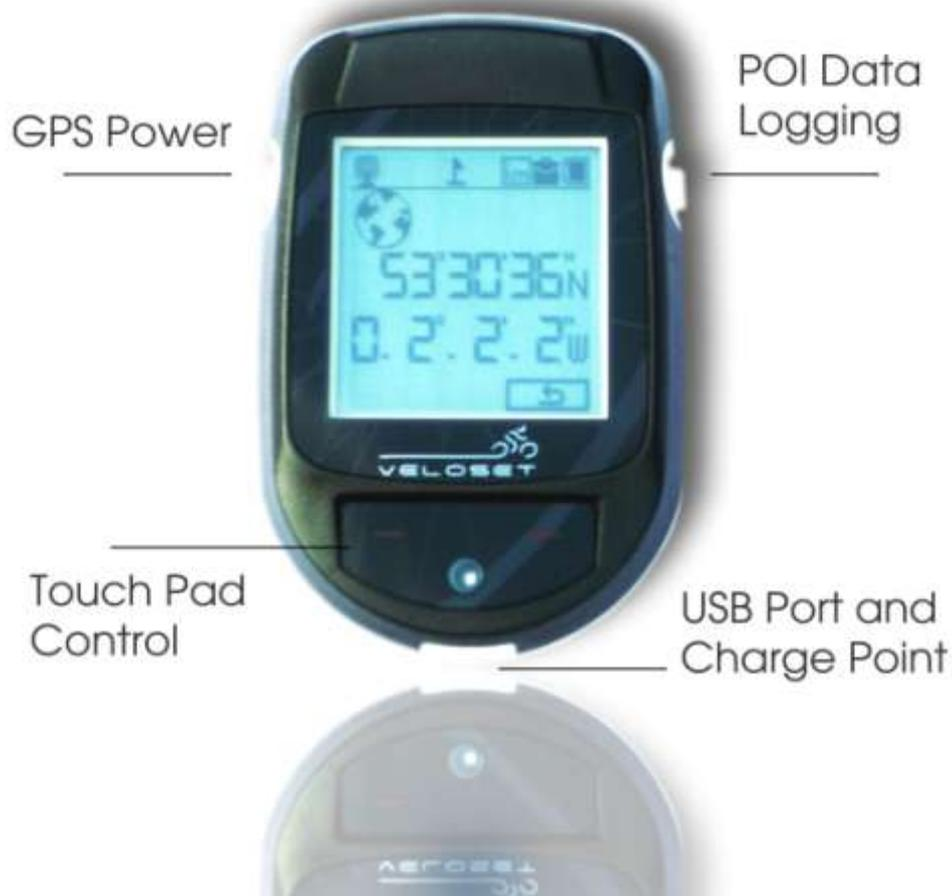
1. GPS Power – Press for 1 second to turn ON. Single press to turn back-light on/off. Hold power button for 5 seconds to turn OFF.
