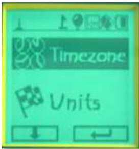
Switch to SET MODE from the main screen menu (left pad) and enter (right pad), press the left button to set the time zone, press the right button to exit.
