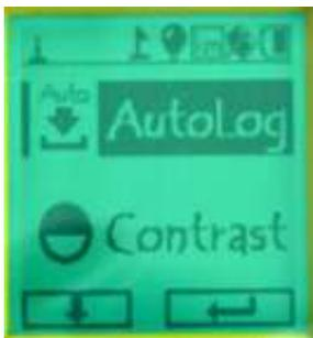
Select auto log and choose on that means the data logger is always on when you switch on device
