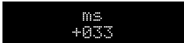
If a frame rate has been set, the reading is also given in frames. Using the same example, with a frame rate of 25 frames the audio is ahead by 0.84 frames.
