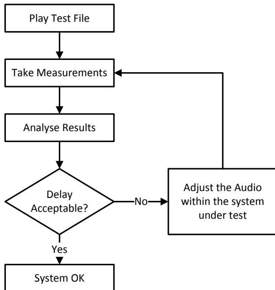
This uses both modes of Sync-One2, Measurement Mode and Menu Mode. Measurement Mode takes the readings and stores the 60 most recent in a memory buffer. Always take a number of readings to determine the error, to smooth out the variances in signal processing.
