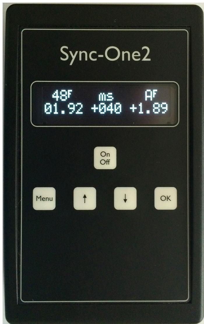
Sync-One2 is an easy to use hand held tool suitable for professional and amateur users to quickly and easily analyse audio/visual synchronisation problems.
