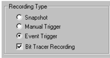
In Bit Tracer Recording, you can use the Snapshot, Manual Trigger, and Event Trigger recording types.
