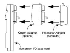
Option Adapters add a time of day clock and one or two additional Modbus ports, depending on the Adapter model. Features of an Option Adapter are configured along with the Processor Adapter; as far as controller configuration is concerned, the division between the two is transparent.
