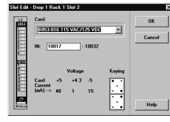
2. Select the card to insert in the slot (selected in the Traffic Cop window) from the drop-down list. Selecting a card displays the power supply loading and mechanical keying for the card.
