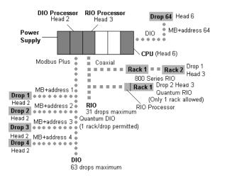
DIO drops connected to a DIO processor occupying Head 2 (slot 2) of the local Quantum backplane. All of those drops belong to Head 2.
