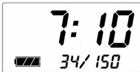
Figure 4: Example of the display on the LCD when the Display Statistics Push Button is pressed and released second time while the backlight is enabled
