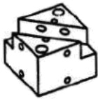
Figure 2. Accelerometer mounts for Q3
