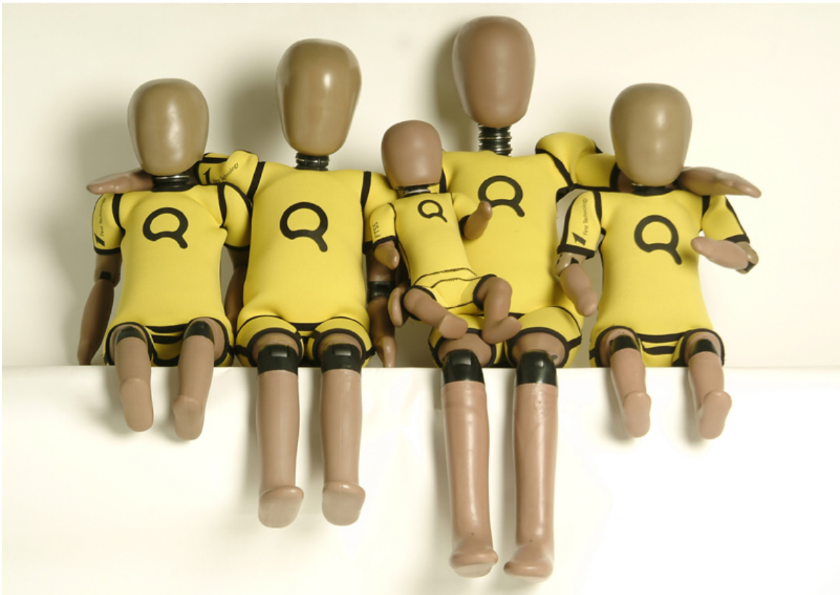
Figure I. Q-dummy family (from left to right: Q1.5, Q3, Q0, Q6 and Q1)
