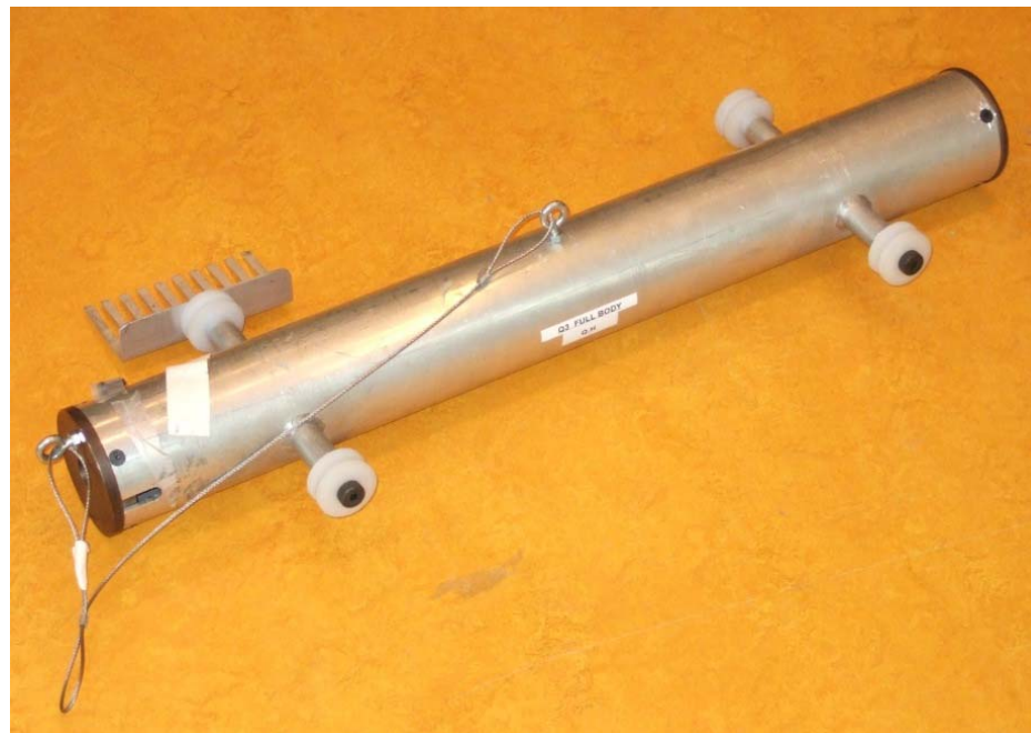
Figure 19. Q3 full-body impactor (accelerometer not shown)
