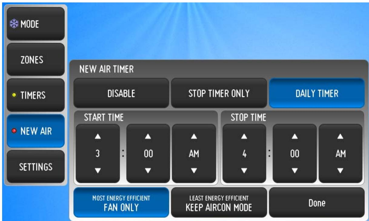
Set the start and stop times using the arrows on screen
