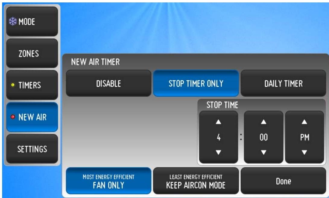
Set the time for New Air to turn off using the arrows on screen
