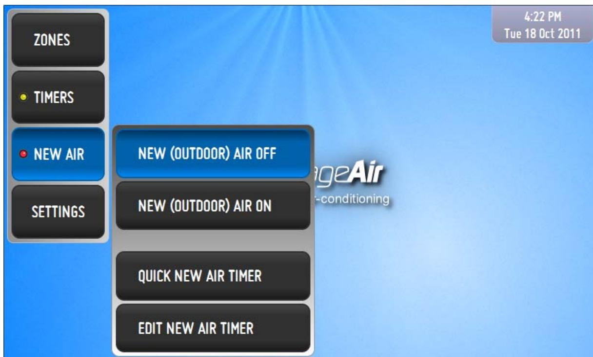
To manually turn on outdoor air, press NEW (OUTDOOR) AIR ON
