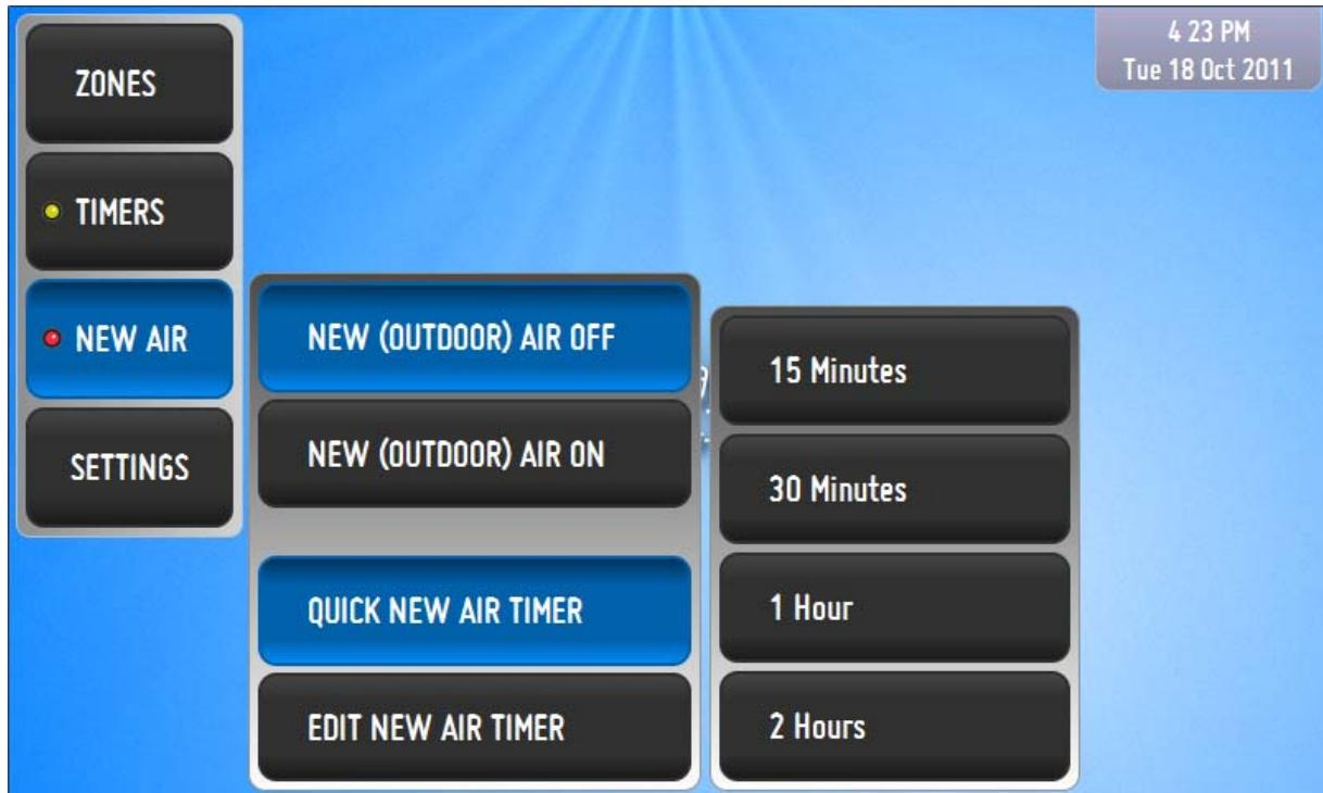
Pressing an amount of time as shown above will enable New (Outdoor) air for the period of time selected before turning off
