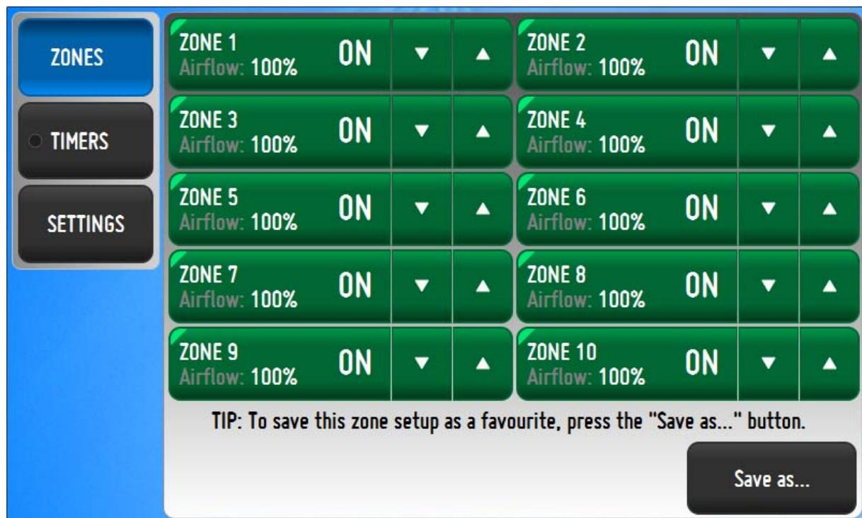
Select the zones to condition, by pressing the zone name or by pressing OFF or ON
