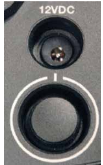
Above photo shows the 12 vdc output connection and On/Off button
