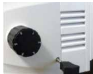
Photo above shows cooling vents on the filter control side.
