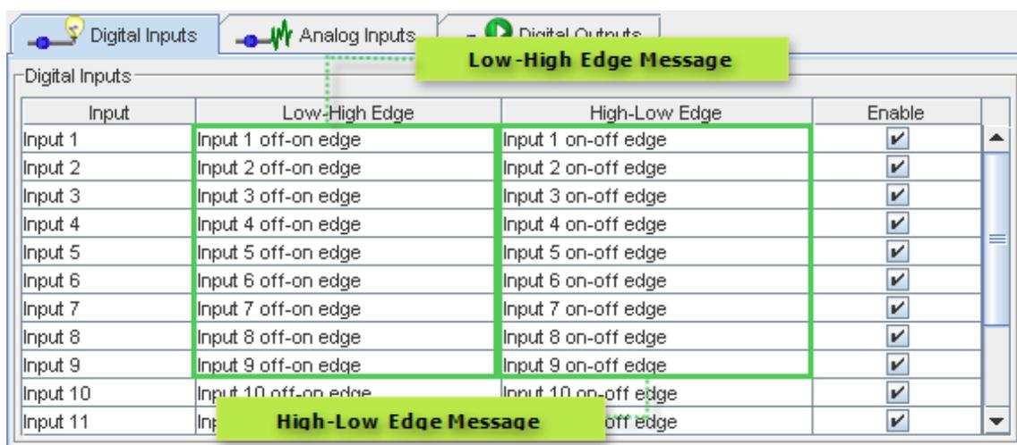
Figure 38 – Configuration of messages of events of digital inputs
