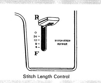
The center portion of this control gives you the means of varying the stitches on the Special Stitch Dial. When the control is turned with the red mark on top the machine sews forward only. When the control is turned with black mark on top the forward designs are varied by machine sewing in a forward and reverse manner. Carefully read directions given in the next section of the book in order to accomplish the various stitches correctly.
