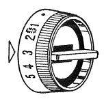
Blind hems are made by using the setting shown above with the Stitch Variegator set with the Red mark on top.
