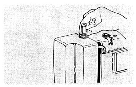
Push down outer ring of presser foot pressure regulator (See above illustration). This will release pressure of presser foot. To increase pressure, push down inner pin until suitable pressure is obtained. For ordinary sewing, the inner pin should be all the way down.
