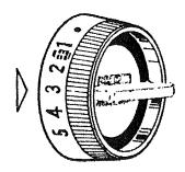
This control must be on the Red Dot in order to do straight stitching. Before turning control, make sure needle is above fabric.
