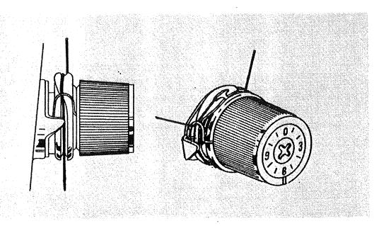
Probably the most important control on your machine is this one that regulates your top thread tension. It consists of discs between which the thread passes. The pressure on these discs is regulated by turning the dial. The higher the number, the tighter the tension.
