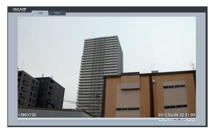
Note: By Default the cameras come with "Installation Mode" set to "ON" to enable Analog output. You must turn installation mode off to use 720p or 1080p streaming.
