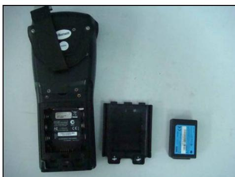
Fig 5-2-3 handheld Psion battery
