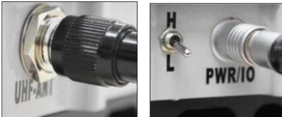
Fig4-2-2 antenna interface and receiver interface
