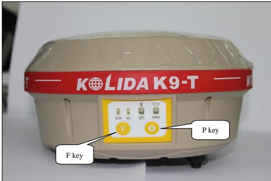
Fig2-1 K9 series mainframe (Rover)
