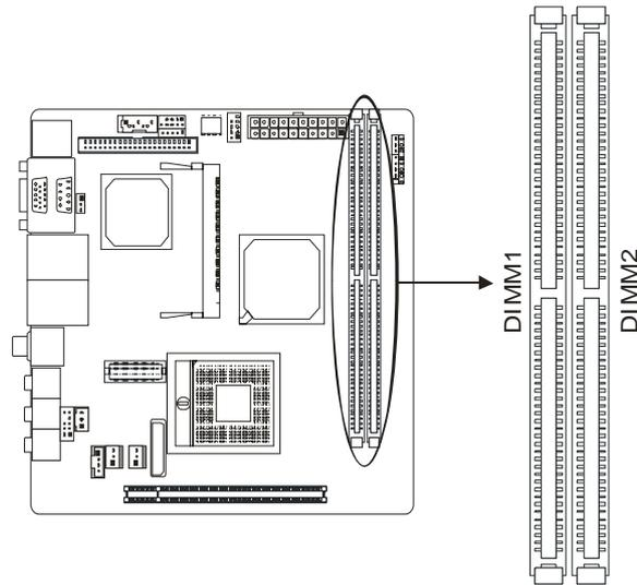
1. Unlock a DIMM slot by pressing the retaining clips outward. Align a DIMM on the slot such that the notch on the DIMM matches the break on the Slot.
