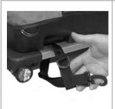
**1.** Attach the parking break strap to the back frame.
