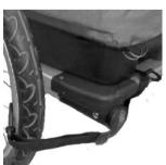
2. Adjust the length of the strap so that you are able to attach the hook to the wheel spokes. Tighten the strap to get minimum movement of the wheel
