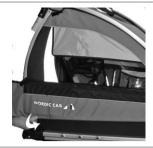
Carefully pull back end of side panel down and under rim of cab. Pull front end of side panel down and under rim of cab.
