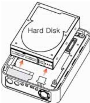
❺ Position the hard drive onto the Enclosure base unit carefully.
