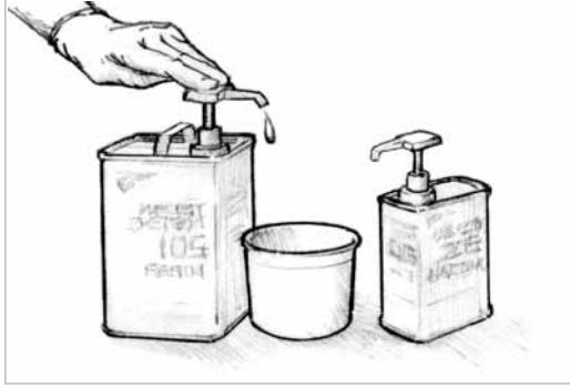
Figure 5-4 Dispense the proper proportions of resin and hardener.
