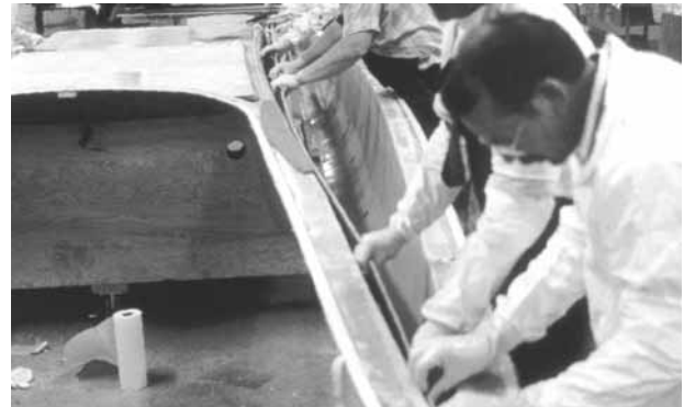
Figure 4-3 After laying in the outer layer of cloth, core materials are placed. Both foam and Douglas fir veneers are used where they are most appropriate.
