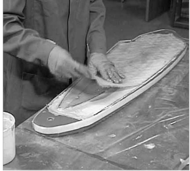
8. Place the wet out fabric in the mold. Squeegee the fabric to remove any air pockets and excess epoxy. Place a layer of release fabric over the laminate. The release fabric will peel off the cured laminate, leaving a fine-textured surface. Excess epoxy which has bled through will be removed along with the release fabric.
