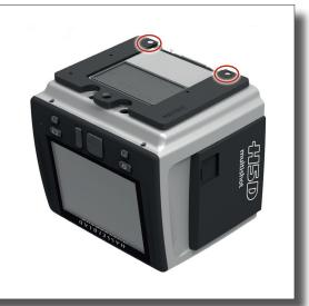
5. The Battery Adapter includes three captive screws. Check for the correct orientation of the Battery Adapter (as in the illustration) and lower it down onto the Battery adapter plate, ensuring the plug A fits firmly into the connector port B. Screw the Battery Adapter onto the Battery adapter plate using the three captive screws. To avoid damage to the components, do not overtighten the screws.
