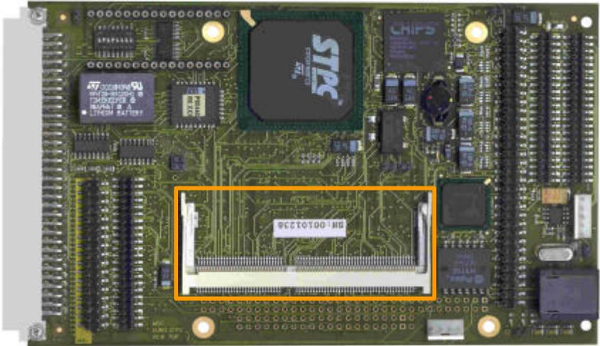
The EURO STPC-I board has a SO-DIMM socket for standard 3,3V SO-DIMM modules (Fast Page Mode or EDO):
