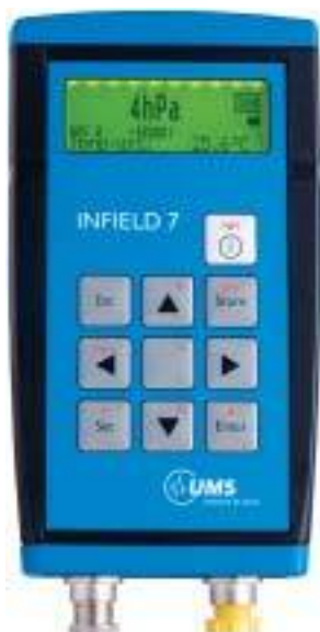
◀ Infield 7 Handheld digital display interfaces with all UMS tensiometers for quick data collection.
