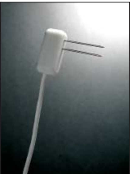
■ SH-1 30mm dual needle length 3 parameters- Thermal Conductivity, Thermal Diffusivity, and Specific Heat.
