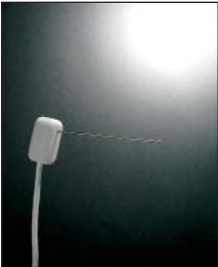
■ KS-1 6cm needle length Thermal conductivity of liquids.
