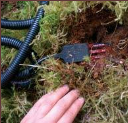
▲ Instrumenting canopy soil over 19 m off the ground.
