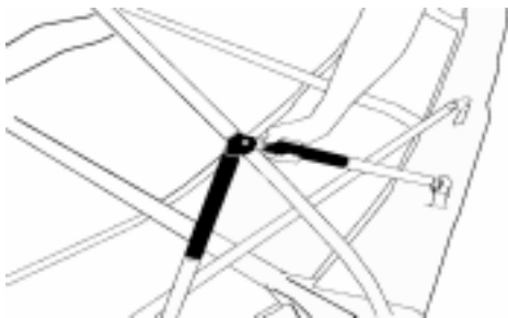
Figure 10. Turn the Y-tubes open one at a time and join them to the boom.
