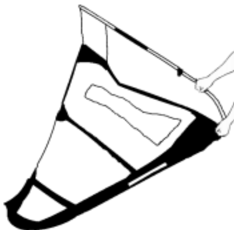
Figure 17. Lift the wing by holding from the boom.
