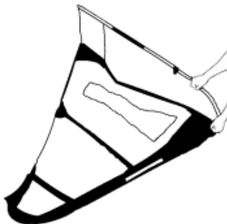
Figure 13. Lift the wing by holding from the boom.
