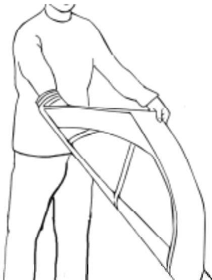
Figure 19. You can tighten up the roll by pushing one hand inside the roll.
