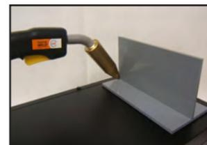
**STEP 4:** Place the tip of the gun on the weld line on the far LEFT edge of the coupon. This is position 1. Hold the gun at a 45° work angle and a 0° travel angle. Pull and release the trigger.
