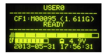
The name of the active profile is shown in the first line. The full profile data will be displayed if the ENTER key is pressed.
