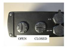
An external 6 V battery (5.5 V - 8 V DC is acceptable) can also be connected to the DC jack using a cable available from Pettersson. The Main Power switch (INT/EXT) is used to select internal or external supply or to disconnect power (mid position).
