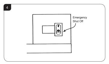
(This switch is set to be ON (I) during normal operation and must remain ON)
