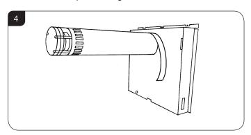
2.9 Place the sealing ring over the flue and position it up against the rear of the appliance. See Diagram 5.
