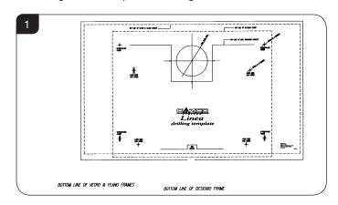
2.4 Having ensured that the template is level, mark the centre of the flue hole and the position of four fixing holes for the wallfixing bracket. See Diagram 2.
